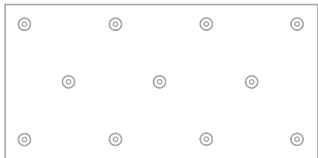
Figure 6 Fastener pattern (11 No. per board) Board size to 2400 mm x 1200 mm - 3.81 fixings / m 2
