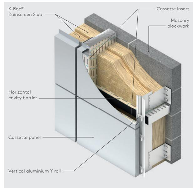
Figure 2 - Aluminium Cassette & Masonry Blockwork
